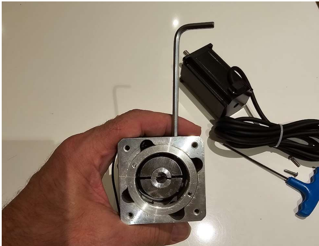
Figure 6 Clean the stepper motor shaft and gearbox shaft coupler with acetone or similar, to limit the chance of slippage between the motor and gearbox. Turn the gearbox shaft coupler such that an allen key fits the bolts. Fit the shaft adapter
