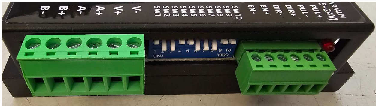
Figure 9 Correct dip switch settings for controller without feedback (Zero position instead)
