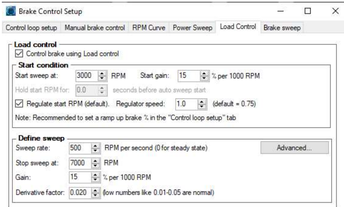
Figure 14 Load Control is the best brake mode for water brakes. Here is a starting point for the settings
