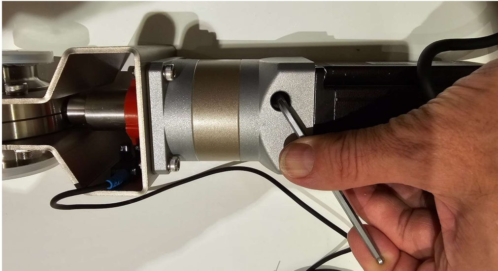
Figure 7 First secure the stepper to the gearbox with 4 x m4 bolts. Then tighten the shaft coupler bolts, a bit at the time, symmetrically on each side. Torque spec is 8.7Nm (6.4 lb ft). Fit the caps to the screw holes to keep water/dirt out
