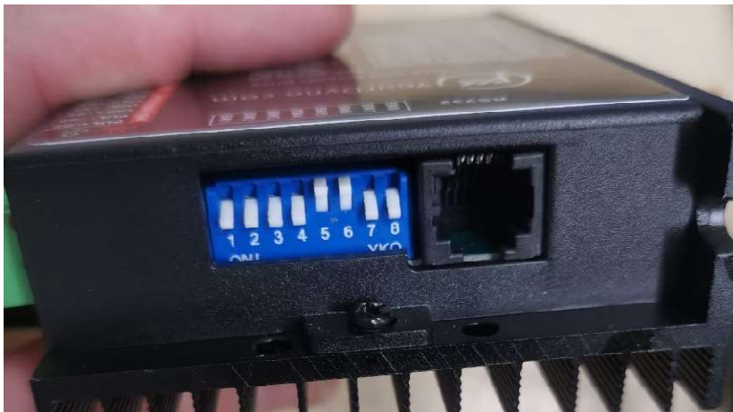
Figure 8 Correct stepper dip switch settings for the controller with feedback
